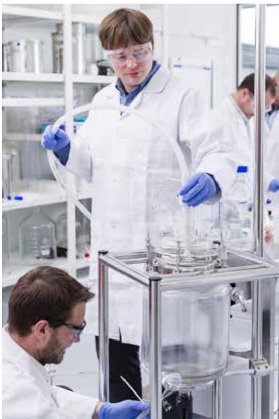
Figure 3: Cleaning mobile glass reactors
